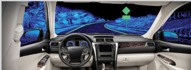
A single lidar sensor generates around 1 Gbyte/second.
