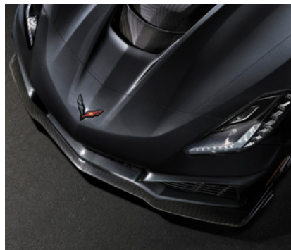
Book-matched carbon fiber elements include the downforce-producing front underwing.
